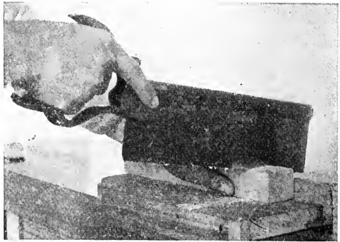
Fig. 71 - Sawing, Third Position
